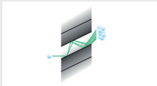
Figure 9: Schematic representation of the electron multiplication in a single channel.
