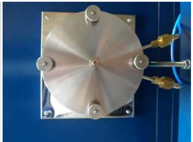
Water cooled flange assembly
