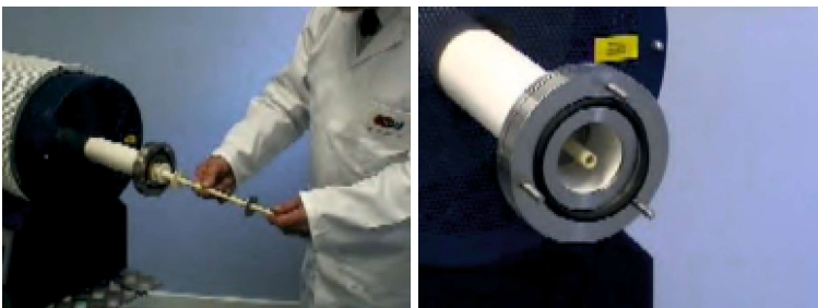
Insertion of the radiation shields in to the work tube
