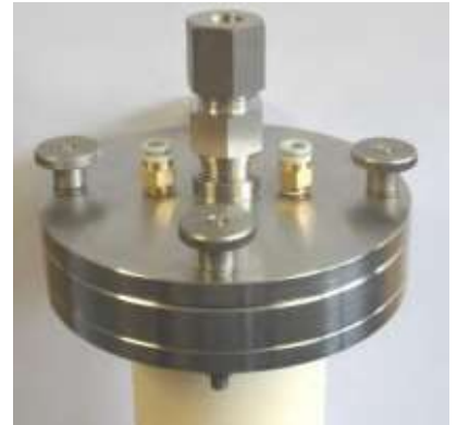
Triple flange end seal with thermocouple gland
