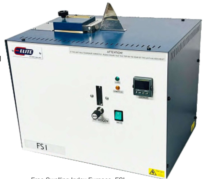
Free Swelling Index Furnace, FSI
