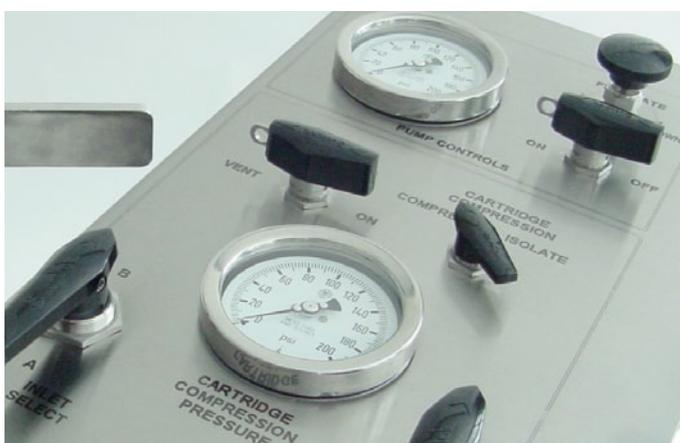
**Figure 18.** The pneumatic control panel located on the top of the flash system frame makes operation easy. The panel is divided into three sections that allow users to control the pumping system, The hydraulic hoist is used to remove the head assembly, insert a cartridge.
