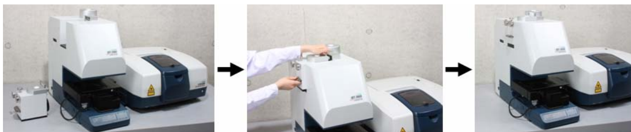
Fig. 1 Detector replacement by using detachable detector unit
