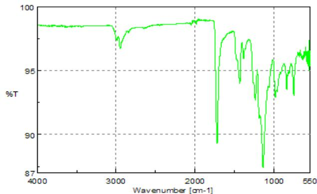
**Figure 6.** Spectrum of the Red polymer found in a taillight.
