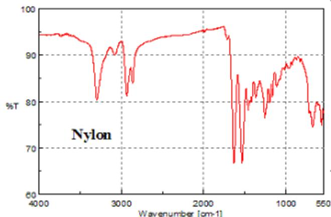
Figure 2. Spectrum from vehicle carpet fibers
