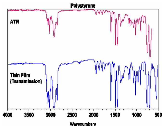
Figure 1. Transmission and ATR spectra of polystyrene.
