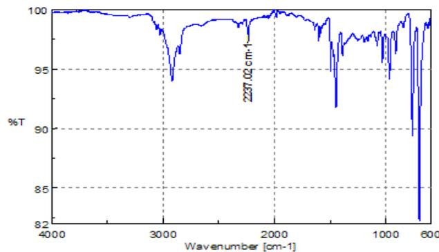
**Figure 7.** Dashboard knobs identified as (80% styrene) Poly(styrene:acrylonitrile)
