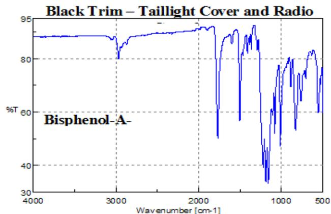
**Figure 5.** Spectrum from the trim around the radio console
