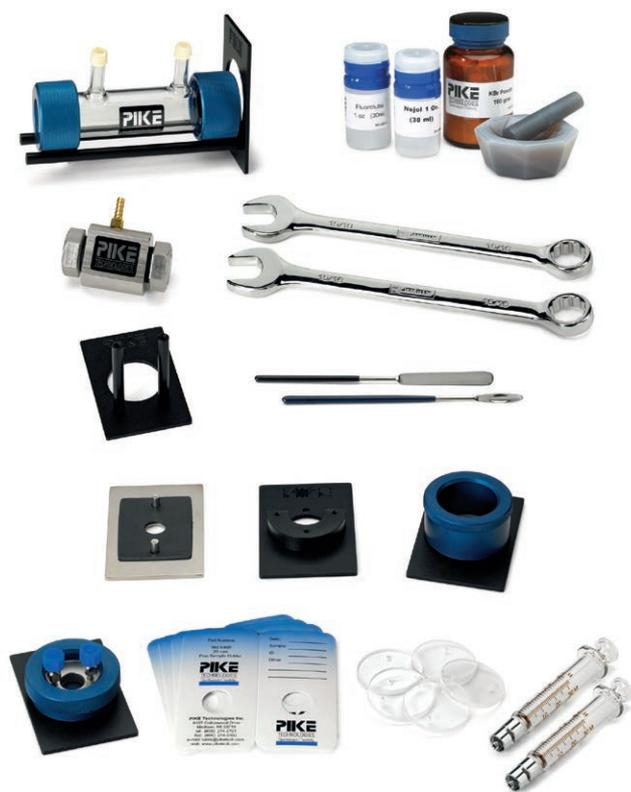
The Educational Sampling Kit contains all necessary tools for the analysis of gas, liquid and solid samples. It was designed as a low-cost alternative for busy teaching laboratories. The kit offers a 100 mm x 25 mm gas cell with straight, septa protected tubes, a bolt press for making KBr pellets and a 35-mm mortar and pestle. Please refer to the table below for the detailed list of all components.
