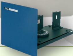
VTA-752 – Film holder (variable incident angle)
