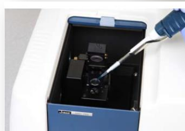
1) Drop sample on the cell
