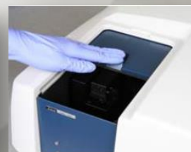
2) Close the cover glass and the lid of sample compartment
