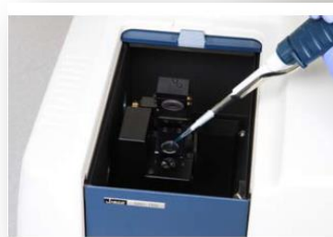
1) Drop sample on the cell
