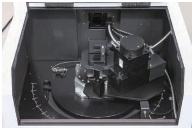
Inside of automated absolute reflectance measurement unit (photo, structural drawing)
