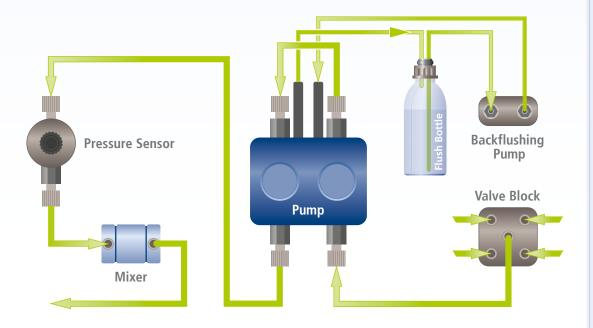
The PN1150 Quaternary Pump is a 1/0.5 stroke double piston pump with a low pressure gradient mixing valve block which is able to generate a gradient mix of solvents from up to four different fluid reservoirs. It works with short piston stroke technology and only two check valves. This results in the low pulsation of a dual piston pump combined with the reliability of a single piston pump. The compensation piston works with a half of the stroke length of the delivery piston.
