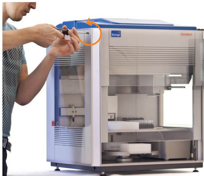
Figure 6. Open the door manually by turning the screw counterclockwise using the T25 Torx screwdriver supplied with the system.
