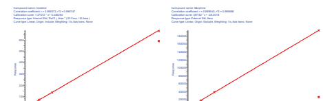
Figures 11-12. Calibration curves of codeine extracted from urine by the 1 mL format and morphine extracted from whole blood by fixed well plate, respectively. Both were produced following Extrahera sample processing.
