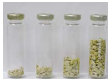
Figure 1: Comparison of 1g, 2g, 4g, and 8g of a HT Polymer Sample in 22mL High Temperature Headspace Vials.
