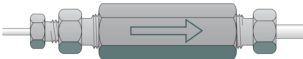
Arrow imprinted on filter body showing recommended direction of flow
