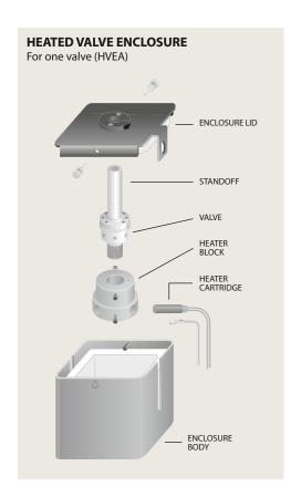
These insulated enclosures allow valves to be operated at temperatures independent of other controlled zones of analytical instruments. The compact construction and minimum power dissipation enable mounting within larger, lower temperature zones without significantly raising the larger oven's minimum temperature or impairing its programmability.
