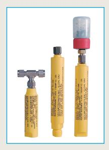
Over 100 different substances are available, including Arsine, Phosphine, and gas phase devices such as CO, NO, and Methane. Available permeation rates range from less than 100 ng/min to 50,000 ng/min. Each G-Cal device is individually calibrated and verified to generate a given mass output per unit time (ng/min) at a set point temperature. A graph which shows an estimated permeation rate vs. temperature from 0 to 50°C is included with each device.
