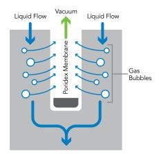
Gas bubbles are actively removed from a flowing liquid stream by vacuum via the PORIDEX membrane.
