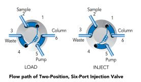
The purpose of an Injection valve is to introduce a sample into a flowing stream of liquid. Some Switching valves become Injection valves by the addition of a Sample Loop (a defined length of tubing and fittings configured to match the angle of the valve ports). Sample is loaded and held in the loop until injection is triggered, either manually or automatically.
