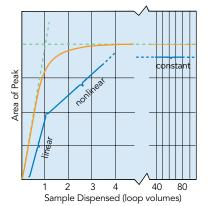
Figure 2 Sample mass (observed peak area) vs. volume of sample dispensed from the syringe, in units of loop volumes, injected onto the column from our dual mode injector such as model 7725
