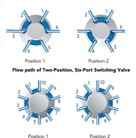
Flow path of Two-Position, Ten-Port Switching Valve
