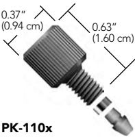
PK-110x 10-32 PK Fitting shown with PK-100x for 1/16" OD tubing
