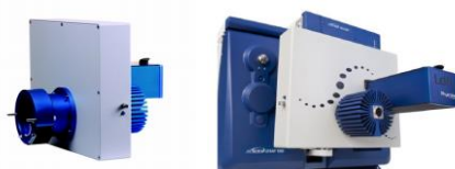
Figure 4: LDTD source design for AB Sciex instrumentation
