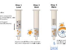
**Figure 1.** Schematic of ISOLUTE® SLE+ Supported Liquid Extraction Procedure.
