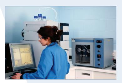
mixed stationary and mobile phases. The second option is based on a quaternary pump which allows on-demand, automated mixing of both stationary and mobile phases. Dynamic Extractions is also able to fit its HPCCC instruments into existing liquid chromatographic systems with these pump configurations.
