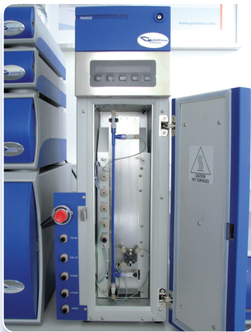
HF-28AN - Analytical HF5 Cartridge with Adapter Plate mounted into AF2000 Thermostat
