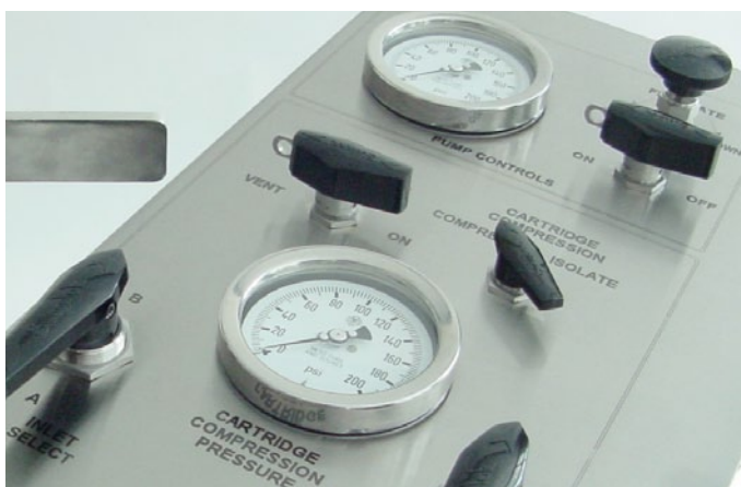
Figure 18. The pneumatic control panel located on the top of the flash system frame makes operation easy. The panel is divided into three sections that allow users to control the pumping system, The hydraulic hoist is used to remove the head assembly, insert a cartridge.
