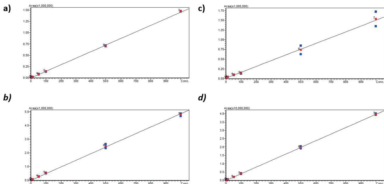
**Figure 4.** Calibration curves for Burprenorphine (a), 6-MAM (b), BZE (c) and Methamphetamine (d) extracted from human nails using the 400  $\mu$ L capacity column format loading 400  $\mu$ L of extract (manual processing). Similar results were achieved for the 400  $\mu$ L capacity plate formats, and for automated processing procedures.
