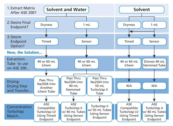
With many labs adapting the new methodology using the Dionex ASE 200 system, Biotage has recognized the need to assist laboratories with their concentration options.
