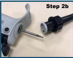
2) Using the calibration tool, insert the wide end into the 2 slots of the cap on the plunger assembly. Rotate it, at the base, counterclockwise to unlock and remove the cap.
