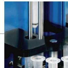
Positive pressure, stepper motor syringe pump delivers precise flow rates.
