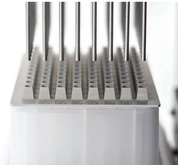
Biotage® ACT (Anti Cross Talk) plate adapter is a novel (patent pending) solution to the phenomenon of hot spot cross contamination, or cross talk, during evaporation in 96-well plate based assays. The simple but effective design prevents cross talk on evaporation when using the Biotage® SPE Dry 96, decreasing the risks of falsely elevated results, which would otherwise compromise analytical results. See page 83 for further details.
