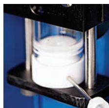
Closed fluid path system with segregated waste lines maintain integrity of sample.
