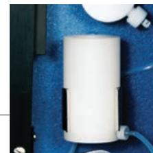
Reagent mixing chamber allows automated online reagent blending in the method.
