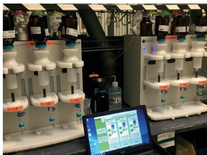
**Figure 1.** Two Biotage® Horizon 5000 extractors equipped with carbon cartridges for extraction. Both extractors are controlled using the PC in the middle of the image.**Table 6.** Initial demonstration of accuracy (IDA).
