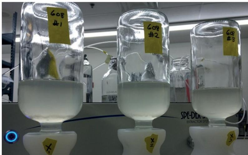
Figure 1. Shows synthetic wastewater being extracted with the SPE-DEX 5000. Note the particulate in each sample.
