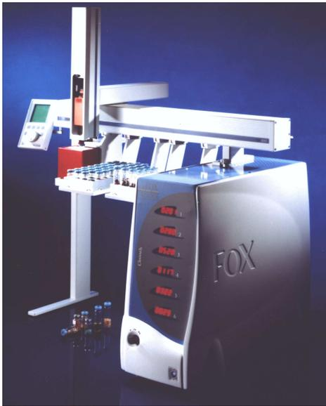
As shown, The Fox 3000/4000 with the HS100 OdorScanner Autosampler. The autosampler is configured with 2\*32 Position trays designed to accommodate either 10-ml sealed vials or 20-ml vials. An Integrated Heating module conditions the samples according to a time and temperature program. Conditioning temperature ranges from 30°C to 150°C. The sample may be agitated while heated to insure repeatable sampling conditions.
