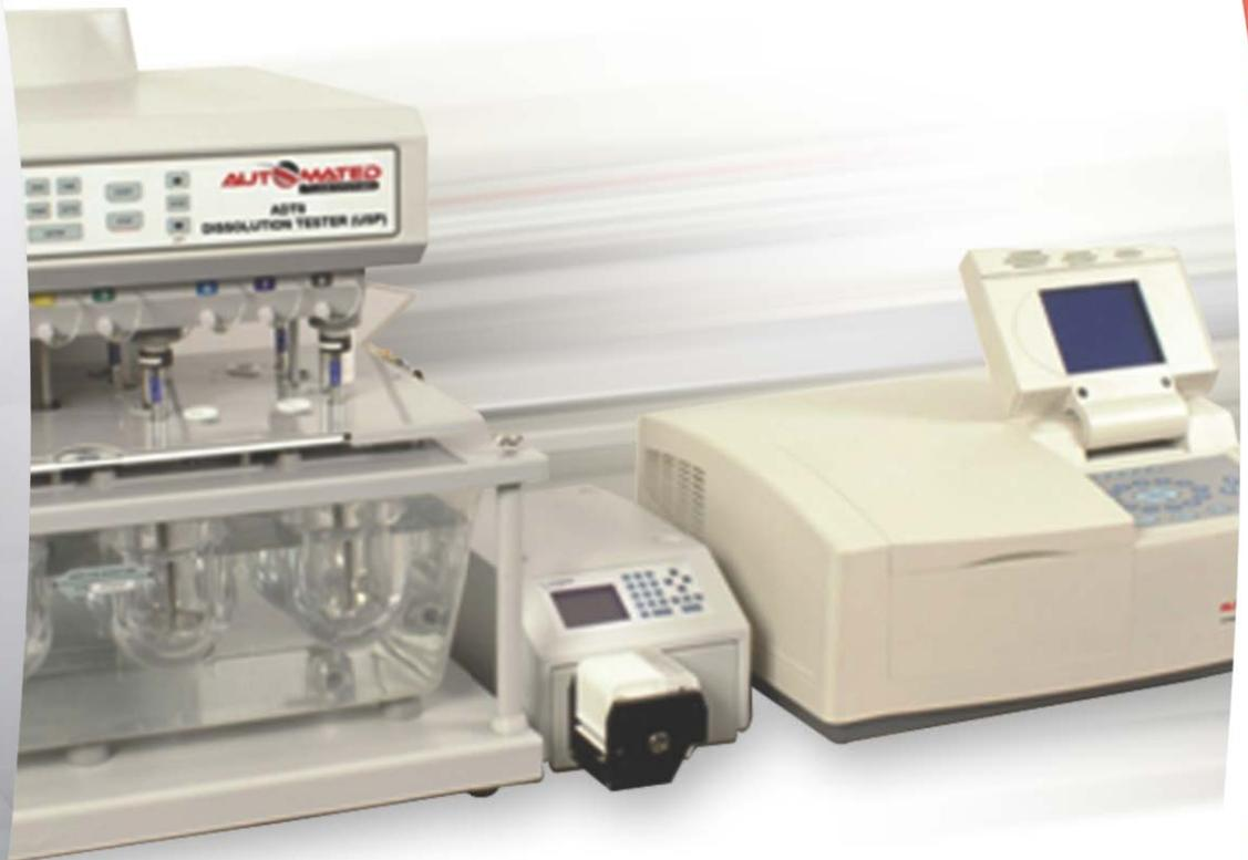
This application is used to automate testing of Tablets, Capsules and other solid dosage forms according to USP <711> Method 1 and 2 USP <711/724>, EP(European Pharmacopeia) 2.9.3/4> JP(Japanese Pharmacopeia) <6.10>.
