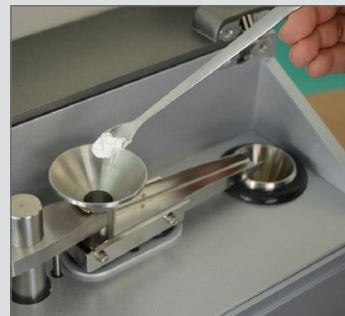
Figure 6 BT-902 open with dry feeding system
