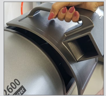
Figure 7 Easy change of the dispersion unit
